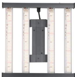
Model:GH-GLG120-A01 Power:120W PPE:288±5% umol/s PPFD:800mol/m 2 /s @30cm
